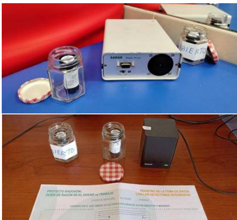
Figure 34. Examples from one citizen scientist of their jars containing CR39 detectors and their continuous measurement equipment at their workplace.
