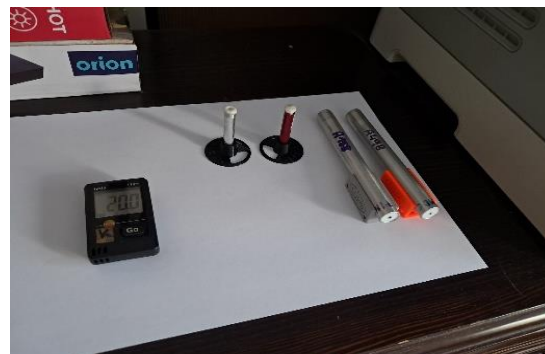
Figure 5 – The SURO (right) and the PentIAQ emission sources used
