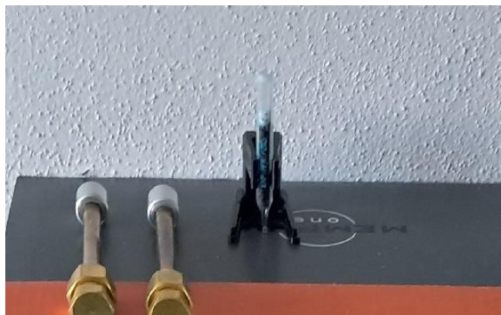
Figure 4 – The SURO (left) and the PentIAQ air samplers used
