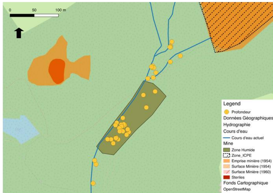
Figure 9. Drilling locations used to assess characteristics of the soil layers in the Rophin watershed (Courtesy of SUBATECH).
